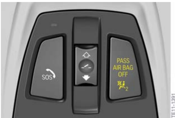
F30 Roof function center with indicator lamp for front passenger airbag deactivation
